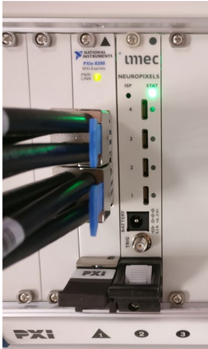
Figure 24: Global status LED of the PXIe acquisition module switching from red to green after correct installation.
