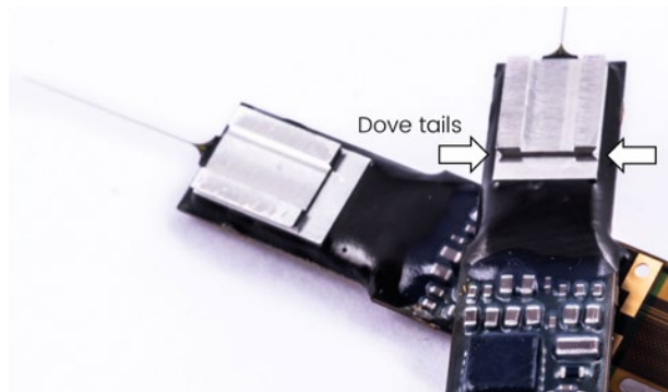
Figure 9: Probes with aluminum cap featuring dedicated dovetail structures.
