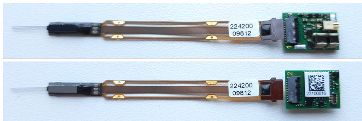
Figure 32: Correct way to plug the flex in the ZIF connector. Top: front side dock, Bottom: back side dock
