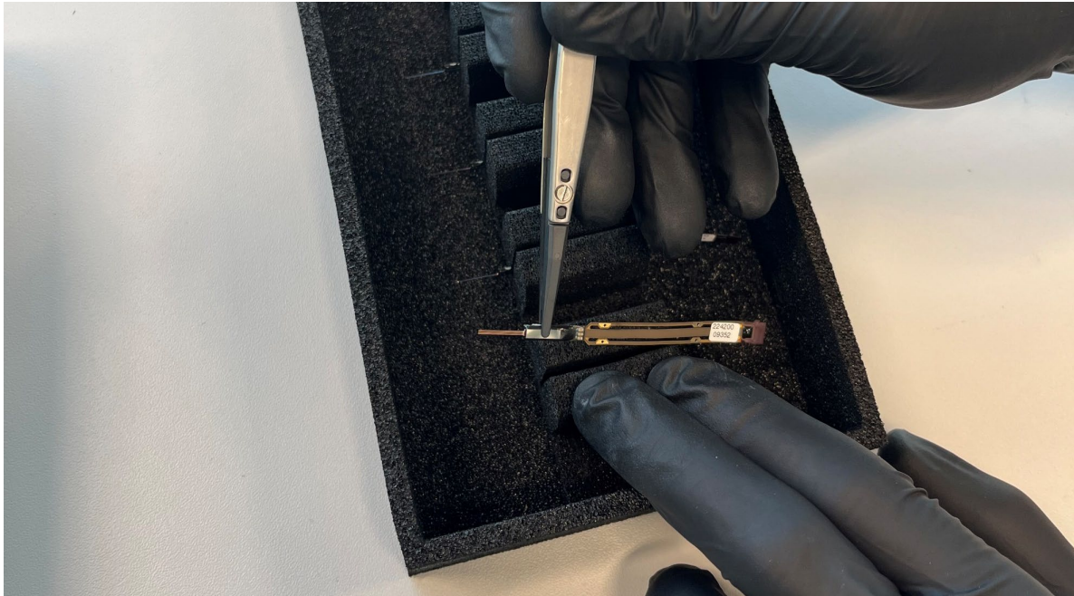
Figure 41: Removing the probe from the foam by clamping the base with tweezers.
