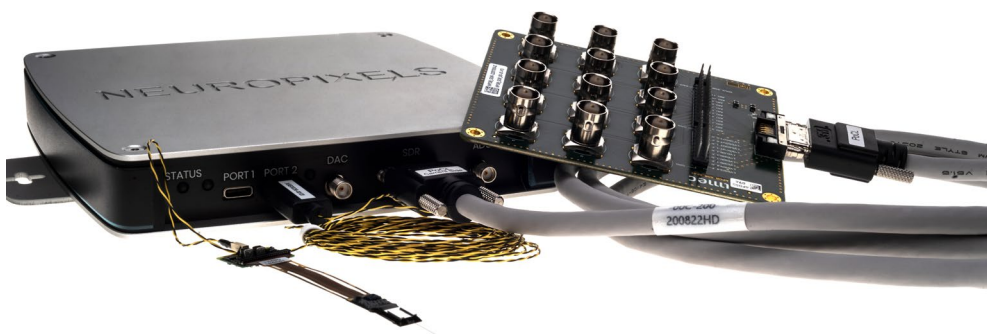
Figure 1: Neuropixels OneBox with breakout board and SDR cable, and a plugged-in neuropixels 1.0 probe
